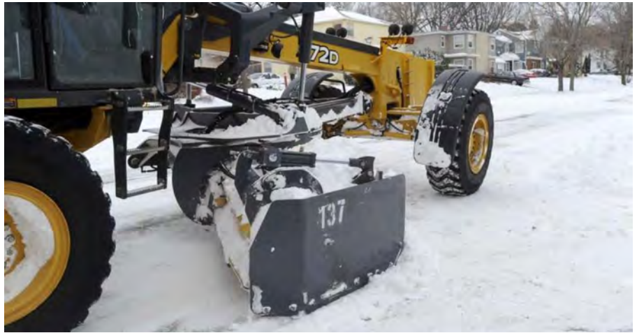
Figure 11 and 12: Curb ramps and pedestrian push buttons should be cleared after snowfall. Some agencies use snow gates to keep curb ramps and driveways clear of snow during plowing. (source: Walk Boston, left; Argus Leader, right)
