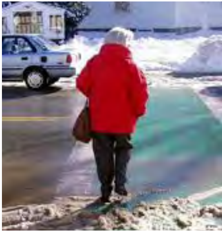
Figure 11 and 12: Curb ramps and pedestrian push buttons should be cleared after snowfall. Some agencies use snow gates to keep curb ramps and driveways clear of snow during plowing. (source: Walk Boston, left; Argus Leader, right)
